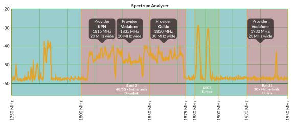
This example illustrates a challenging RF environment where a Dutch telecom provider is transmitting 4G LTE signals very close to the DECT frequency band, leaving only a narrow 5 MHz gap between them. As a result, the DECT antenna becomes overstimulated, preventing it from properly receiving signals across the full DECT spectrum.
