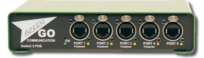
The Green-GO Ethernet switch 5 has been designed specifically for linking a Green-GO communications system into an existing Ethernet network, and to provide a Power Over Ethernet supply to Green-GO outstations.
