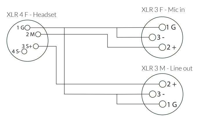
Do not connect pin 1 and 4 on the 4 pin connector For a Wireless beltpack, to remove the DC ofset add a 10uF capacitor between pin 3 of HS and pin 2 of line out
