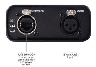
The 2W Slim Audio Interface links 2-wire analogue intercom systems into the Green-GO digital Ethernet network. The 3-pin XLR port will connect to the partyline system. The port can be configured through the setup menu. One of the channels on the partyline system then becomes a group on the Green-GO system.
