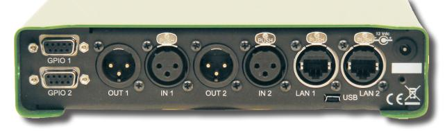
This 4-wire, audio in/out interface with contact closures connects to an existing matrix or other analog interfacing products (program audio in / announce out).
